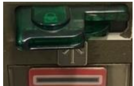
An unusual card reader installed at the card slot
